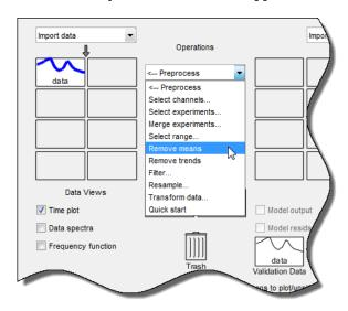
This action adds a new data set to the System Identification app with the default name datad (the suffix d means detrend), and updates the Time Plot window to display both the original and the detrended data. The detrended data has a zero mean value.
